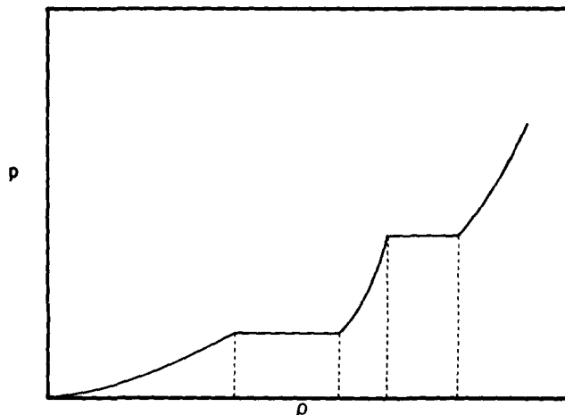
FIG. 1. Relation between the pressure and the number density at a given temperature.
